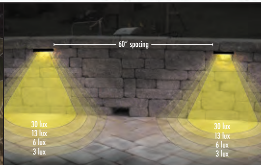
IL6.xxx installed under stone cap
