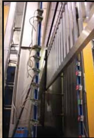
**STEP #10:** Powder application is automated. Compressed process air is dried to -35°F Dew Point for superior adhesion and aesthetics.
