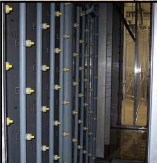
**STEP #2:** Product enters heated alkaline cleaner stage to remove extrusion and fabrication oils.
