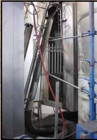
**STEP #8:** A 200 MPH air blast removes water drops from the pre-treated product.
